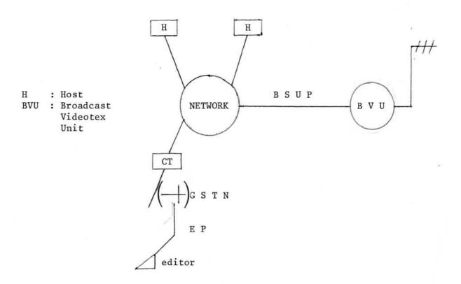
The Broadcast Set Up Protocol (B S U P) between the network and the Broadcast Videotex Unit translates the Editing Protocol (E P) which allows the editor to define the content and properties of the broadcast magazine he is in charge with. EP is an extension of V S A P and B S U P is a specific protocol to access the Broadcast Videotex Unit.
